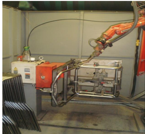
Fig. 1. Robotic arc welding station
