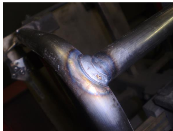
Fig. 6. Completed weld with 16 positions
