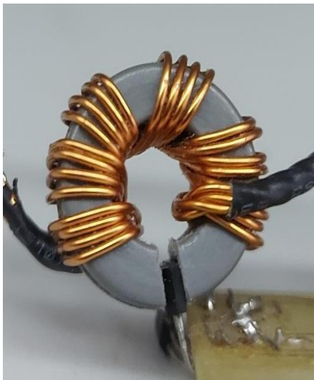
Fig. 3. Hall sensor inside a toroid for amplification of magnetic field
