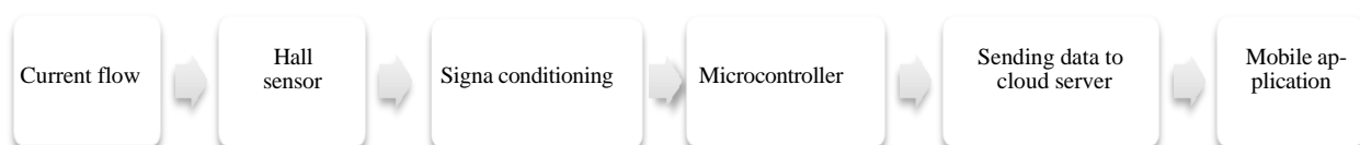
Fig. 2. Development of current measuring device with cloud connection
