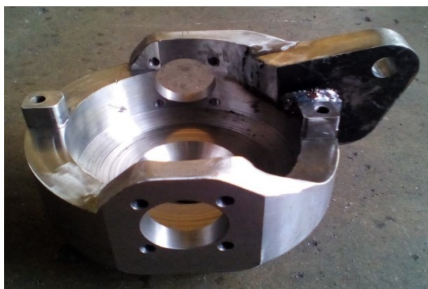
Fig. 13. New mechanical part produced with milling and welding
