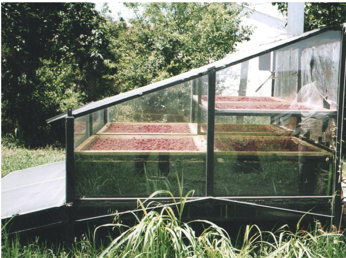
Fig. 4. The disposition of drying shelves (six, 920 × 920 mm) in the solar dryer with water filled vessels
