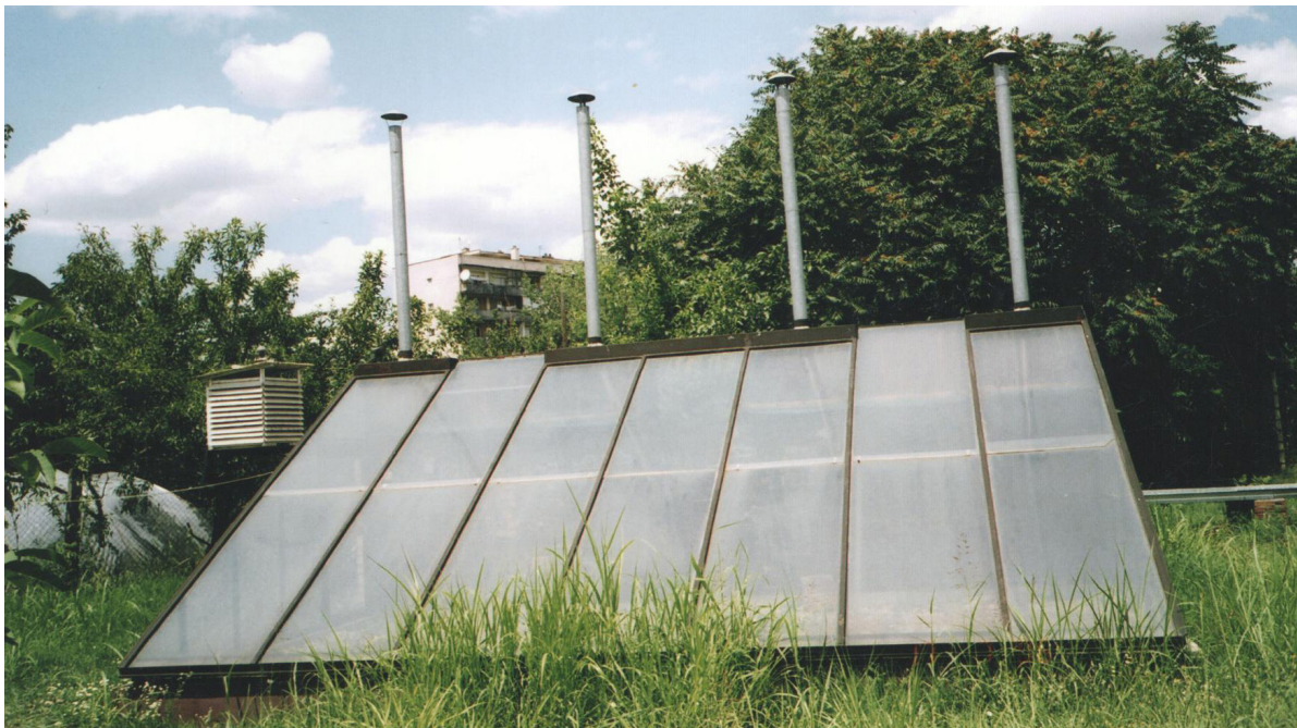
Fig. 3. Solar dryer with rock-bed heat storage
