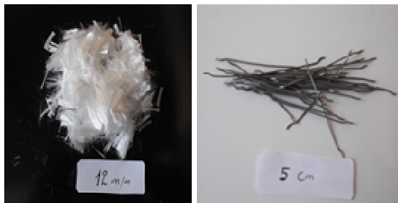
Fig. 3. Polypropylene of length 12 mm and steel fiber of length 5 cm
