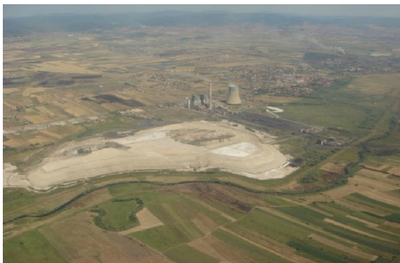
Fig. 2. Deposits of fly and bottom ash from thermo power plants in Kosovo
