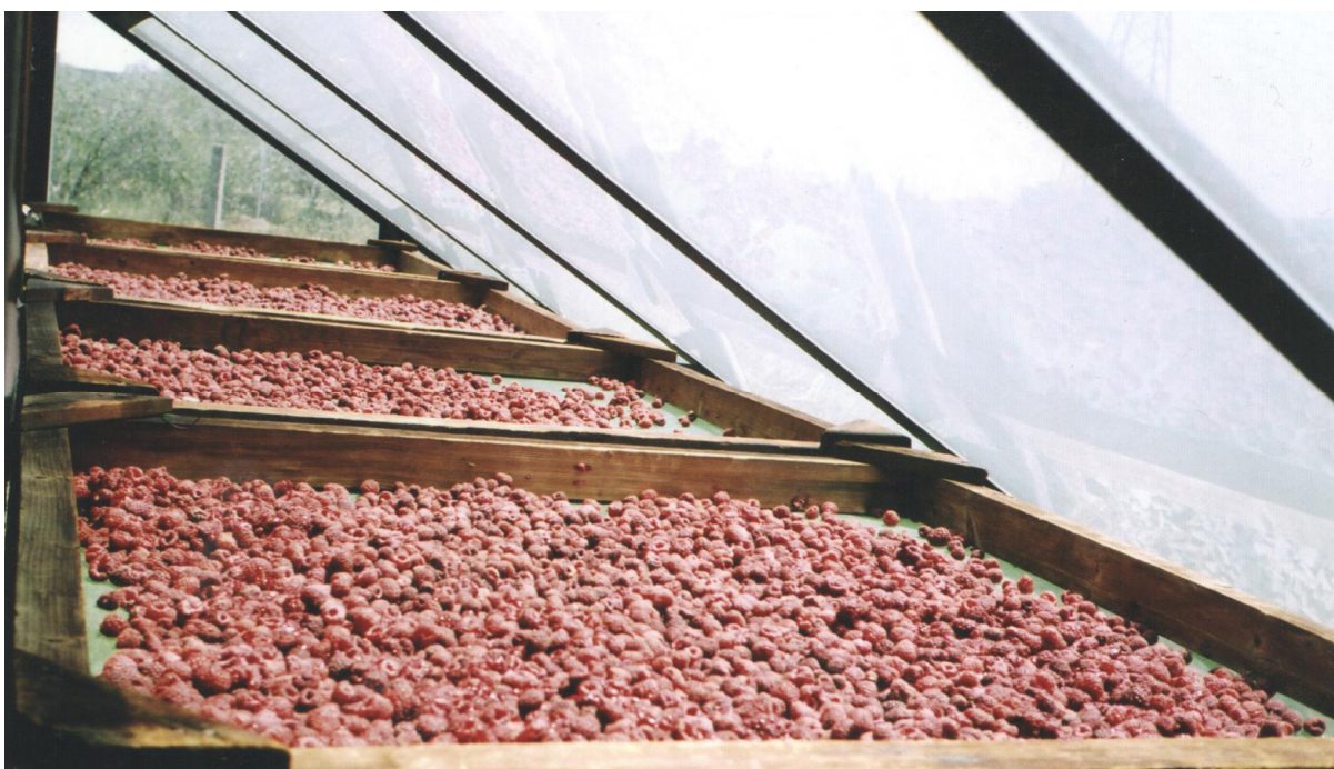
Fig. 5. The disposition of drying shelves (seven, 830×860 mm) in the solar dryer with rock-bed heat storage
