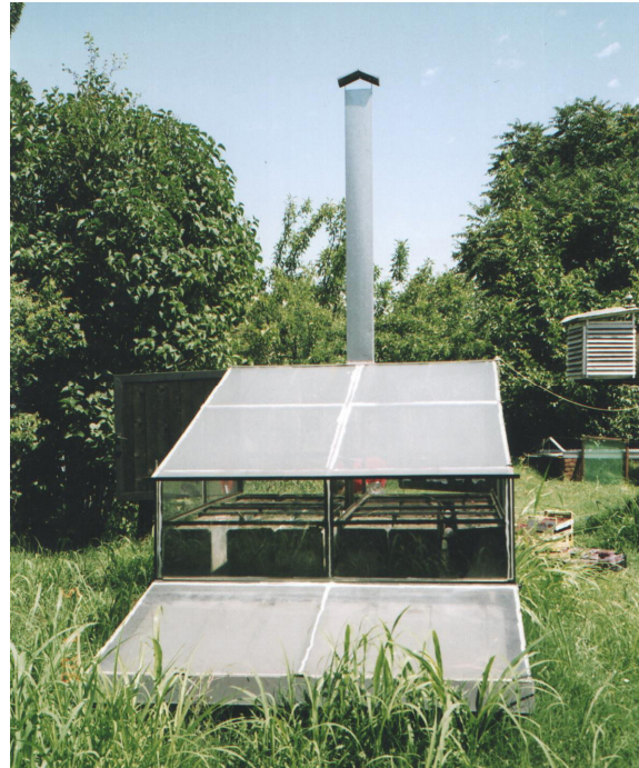
Fig. 2. Solar dryer with water filled vessels
