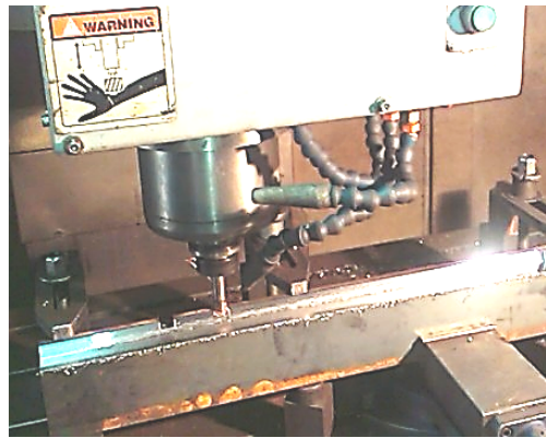
Fig. 6. Milling process on CNC milling center
