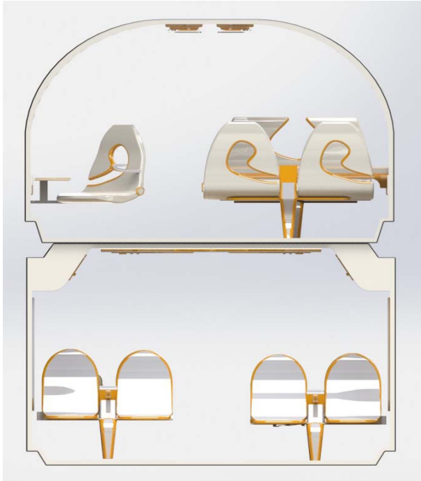
Fig. 13. The cross-section of the double-decker train (Module for clses I and II)
