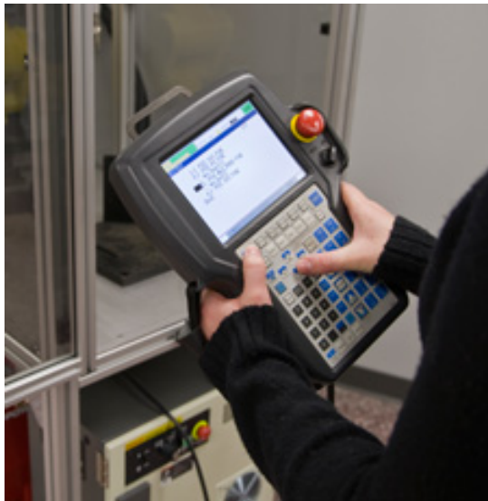
Fig. 4. Simple interactive screen on the pendant.
