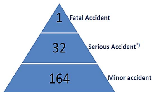
Pyramid 1. Lift users – Number of heavy and slight injuries in respect to a single fatality case.
