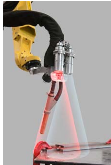
Fig. 5. Welding systems can incorporate vision capabilities that provide for adjusting electrode position and welding parameters to permit quality automated welding even on parts with variations
