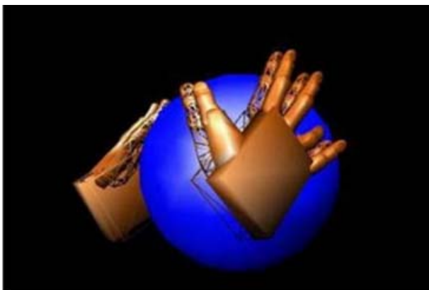
Fig. 4. Holding a Ball with Two Virtual Hands; the Opaque Hands Show the Positions of the Virtual Hands, the Wire-frame Hands Show the Positions of the User's Real Hands. They are, in contrast to the virtual hands, able to penetrate the ball.
