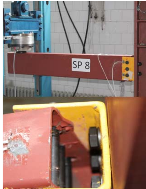
Fig. 20. SP8 model: Collapse of the connection due to plastic deformations of cutting at the end of the beam in the upper long bolt
