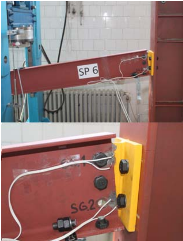
Fig. 18. SP6 model: Connection collapsing due to cutting of lower bolt in the connection of the rib of the beam
