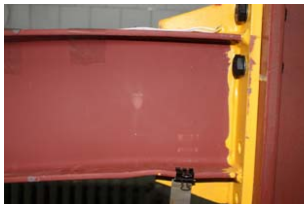
Fig. 13. SP1 model: Appearance of the plastic hinge (stability problem of lateral buckling)
