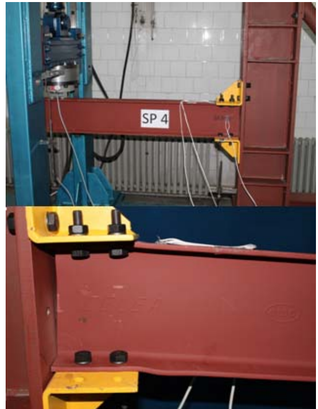
Fig. 16. SP4 model: Appearance of plastic hinge (stability problem of lateral buckling of the lower pressed part of the beam)
