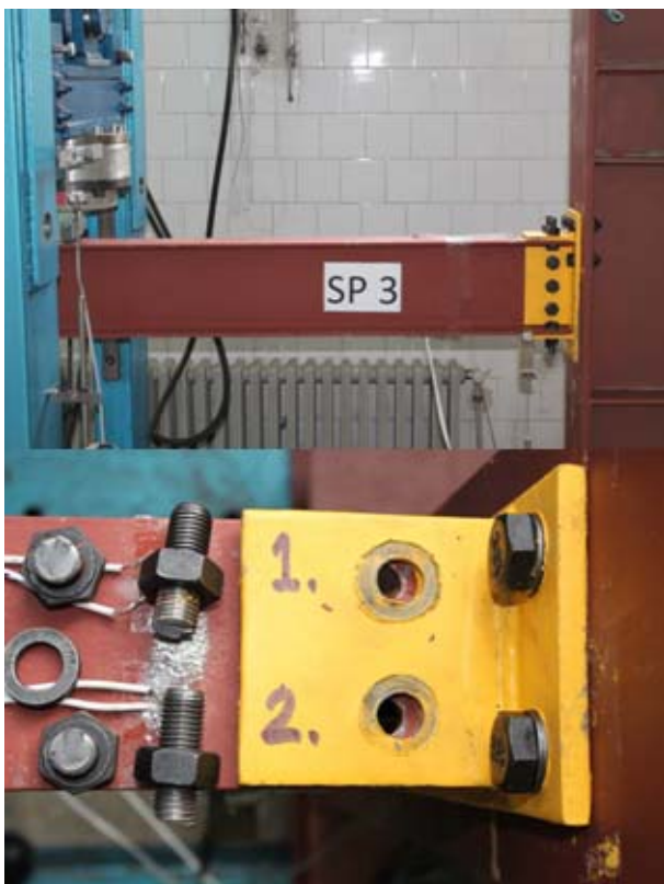
Fig. 15. SP3 model: Connection collapsing due to cutting of the second row bolts in the connection of the upper part of the beam
