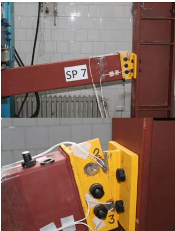
Fig.19. SP7 model: Connection collapsing due to cutting of the upper bolt of the connecting ribs
