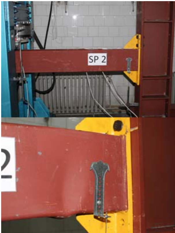
Fig. 14. SP2 model: Appearance of plastic hinge (stability problem of buckling in the lower pressed part of the beam)
