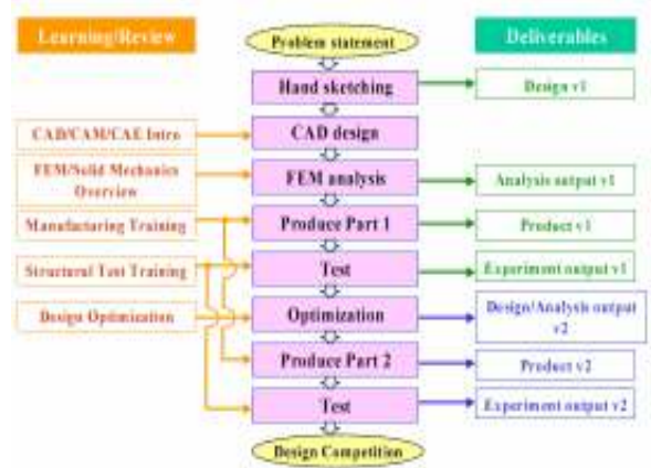
Fig. 10. Flowchart of engineering and rapid prototyping design [11]
