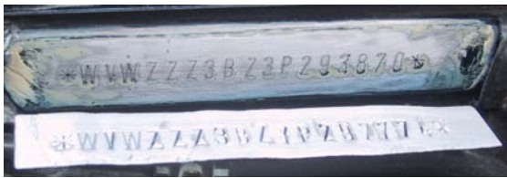
Fig. 18. Originally printed VIN number together with additionally inserted plate
