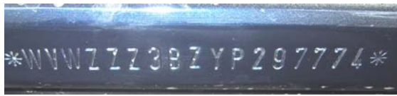
Fig. 17. VIN number of vehicle VW Passat
