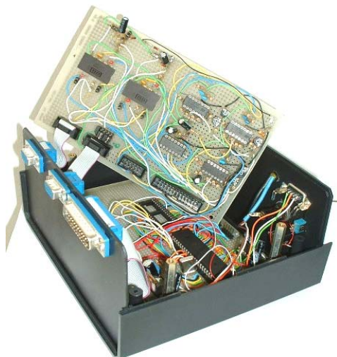
Fig. 7. Prototype version of personal computer interface
