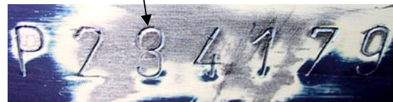
Fig. 16. Original element 3 under the existing element 8
