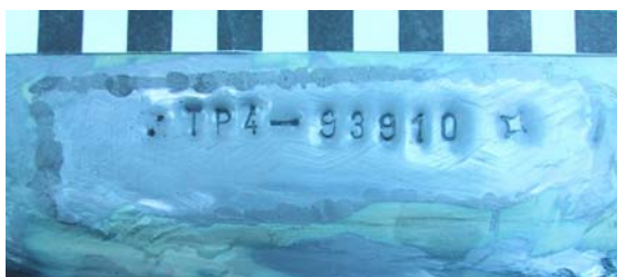
Fig. 14. Closed contour of welded joint around the VIN number
