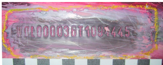
Fig. 13. Closed contour of the welded joint around the VIN number
