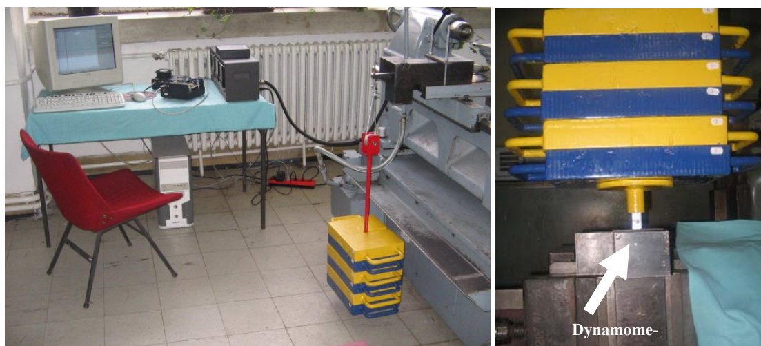
Fig. 19. Measurement system calibration by loading with known force
