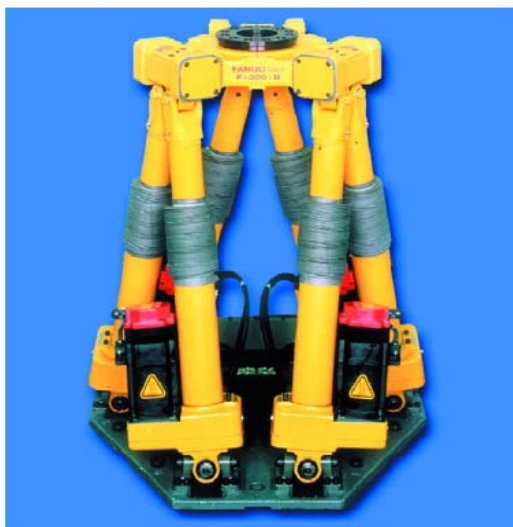
Fig. 1. A Fanuc parallel robot [94] (US patent No. 5987726) [93]
