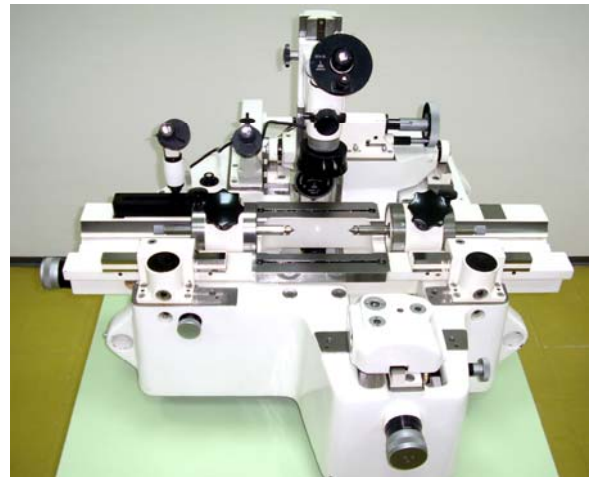
Fig. 2. An aspect of a universal measuring microscope of the model UIM-21
