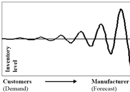
Fig. 1. Inventory variability amplification in a supply chain due to the bullwhip effect
