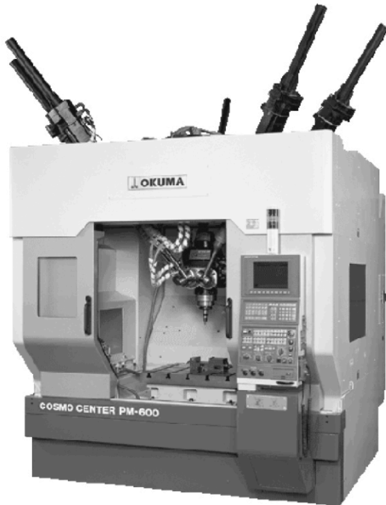
Fig. 15 Parallel mechanism machine tool COSMO CENTER PM-600 [53]
