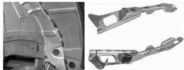
Fig. 4. GSMA brazed parts in car bodies
