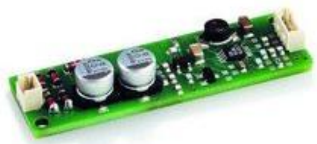
Fig. 3. a) Electronic circuit of PI-E-821.00. b) Energy harvester PI-E-821.00
