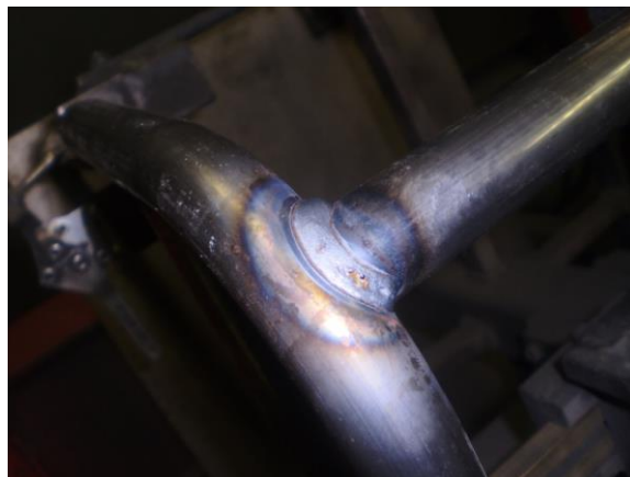
Fig. 6. Completed weld with 16 positions
