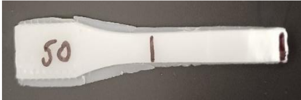
Fig. 10. Flash formation width near the gauge length of the specimen
