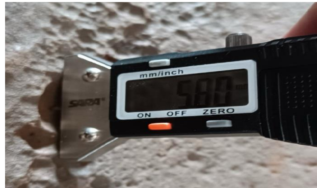
Fig. 8. Damaged location inside the pipe and measured minimum thickness in the damaged segment
