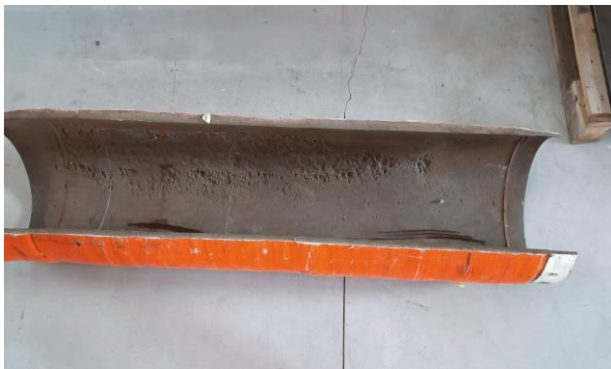
Fig. 8. Damaged location inside the pipe and measured minimum thickness in the damaged segment
