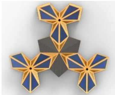
Fig. 8. Pavilion made of 4 connected modules
