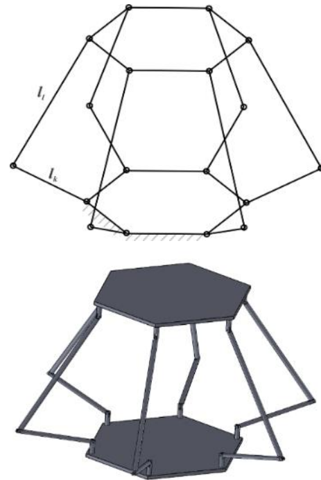
Fig. 4. Manipulator with parallel structure (above) and parallel manipulator constructed in SolidWorks (below)
