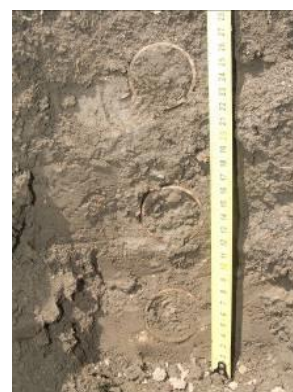
Fig. 4. Placement of the sampling rings on different depth stages
