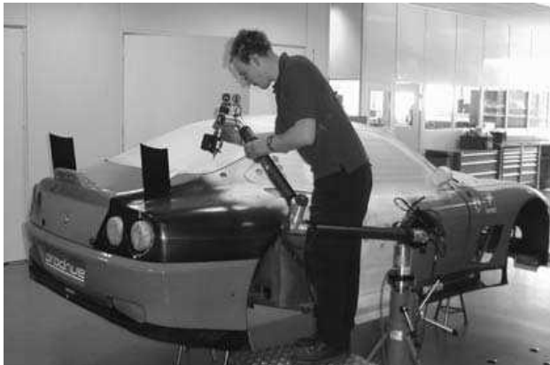
Fig. 2. 3D scanning and computer-aided reverse engineering (CARE) process [3]
