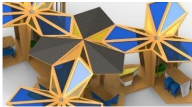
Fig. 9. Roof close-up (solar panels, pipes for rain water collection)
