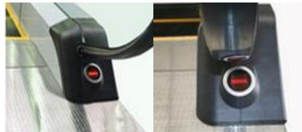
Fig. 9. Emergency stop switch
