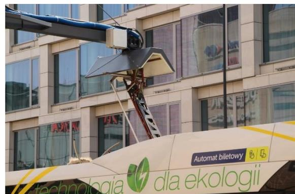
Fig. 3. Pantograph of charging system system Shunk (Kraków, Poland)
