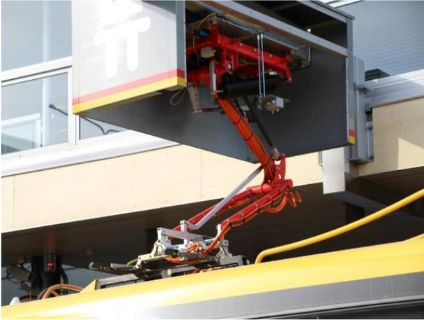
Fig.4. Pantograph of charging system system Opp Charge (Turku, Helsinki)
