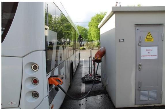
Fig. 1. An example of a plug-in charging system (Bremen)
