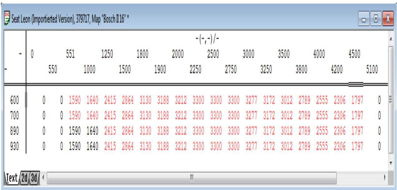
Fig. 5. Modified fuzzy logic map to limit the torque
